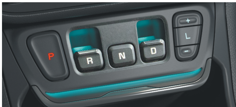
One feature that took some getting used to was the lack of a traditional gearshift. Instead, drivers engage the standard automatic transmission with a series of buttons located below the dashboard LCD display.
